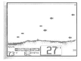
The information collected is controlled by pressing the VIEW button. Pressing VIEW toggles the options "both", "right', "left", or "dwn" (down). When the "dwn" mode is selected, the single 24 degree down-looking element of the Wide Side transducer is used to collect this information. This transducer does not have "wide", "narrow", or "dual" beam options and hollow fish symbols cannot be displayed.
